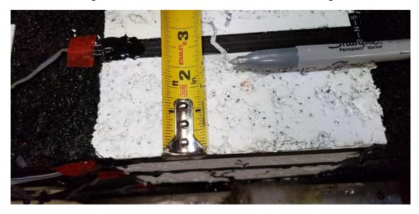
Fig 4 North section surface crack 2 inch from the inner vertical edge
