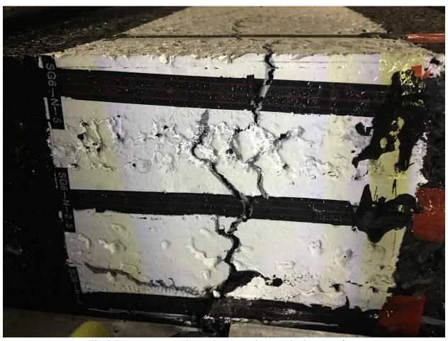
Fig 2 Bottom-up crack north outer edge reached top surface
