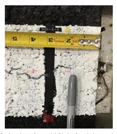
Fig 7 South section surface crack 1.5 inches from the inner vertical edge
