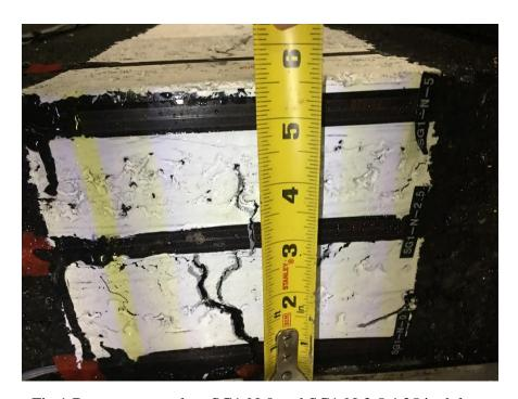
Fig 1 Bottom-up crack at SG1-N-0 and SG1-N-2.5 4.25 inch long
