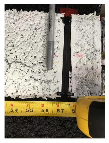
Fig 8 South section surface crack 3.5 inches from the outer vertical edge
