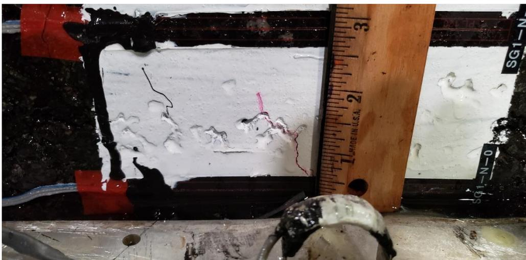
Fig 1 Bottom-up crack at SG1-N-0
