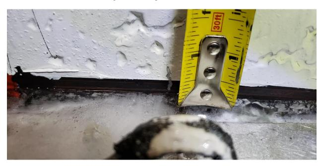
Fig 3 Bottom-up crack at SG1-S-0
