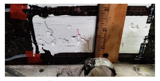
Fig 1 Bottom-up crack at SG1-N-0
