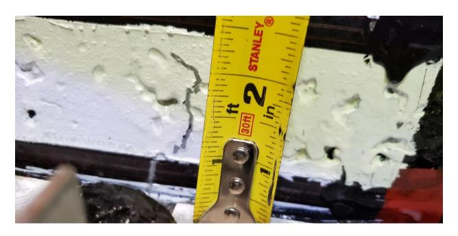
Fig 2 Bottom-up crack at SG6-N-0
