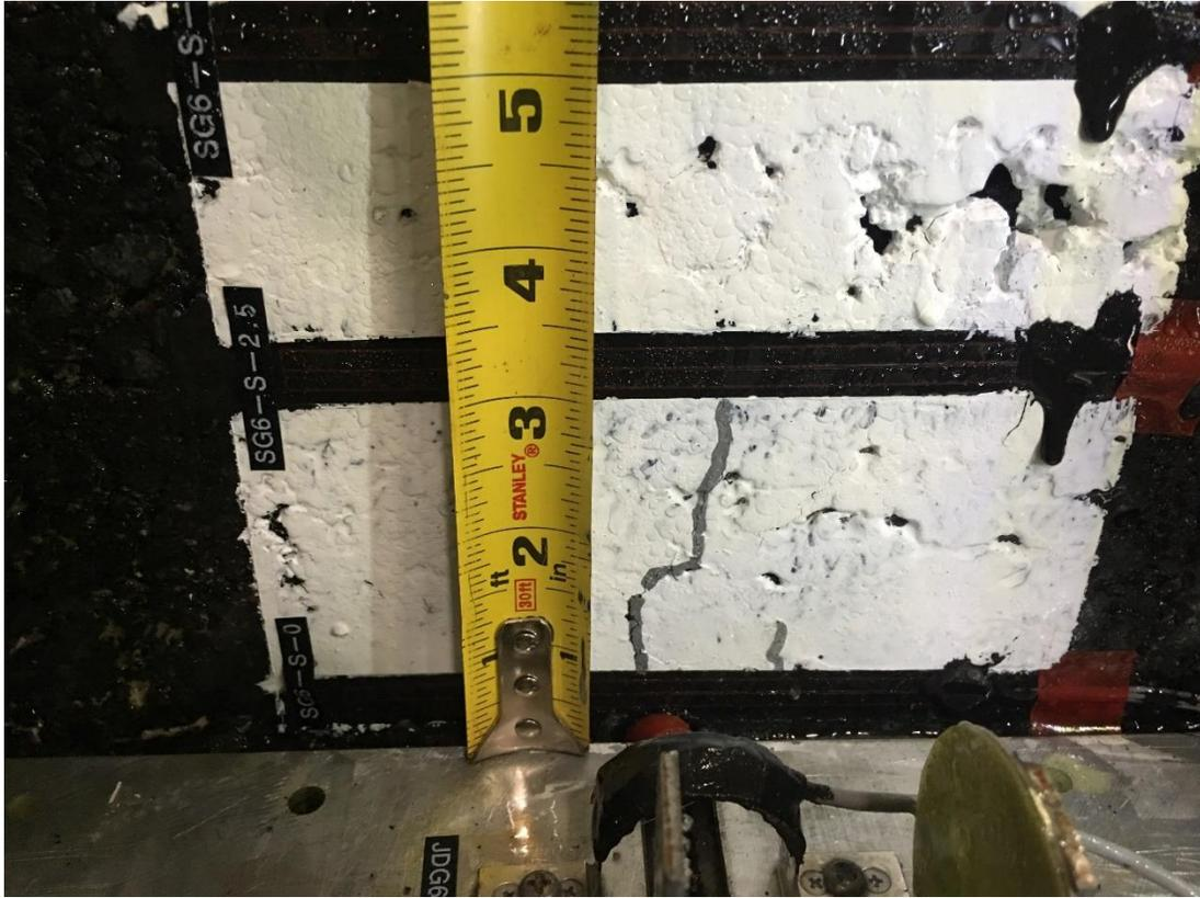
Fig 5 Bottom-up crack at SG6-S-0 3 inch long
