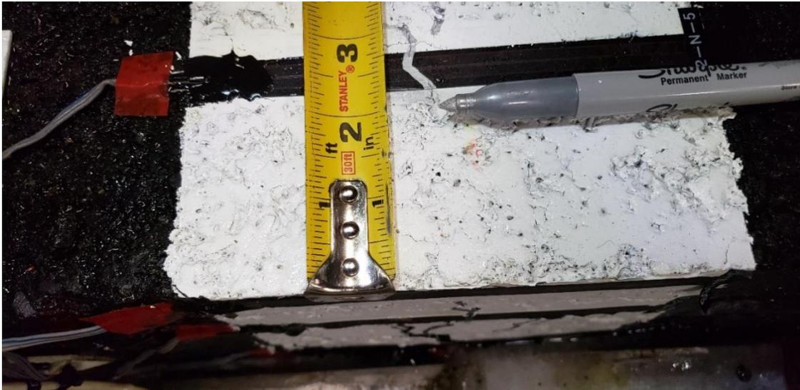
Fig 4 North section surface crack 2 inch from the inner vertical edge
