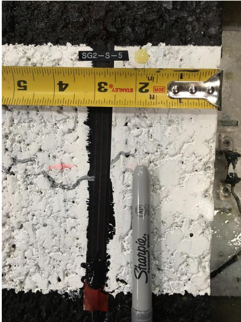
Fig 6 South section surface crack 2 inches from the inner vertical edge
