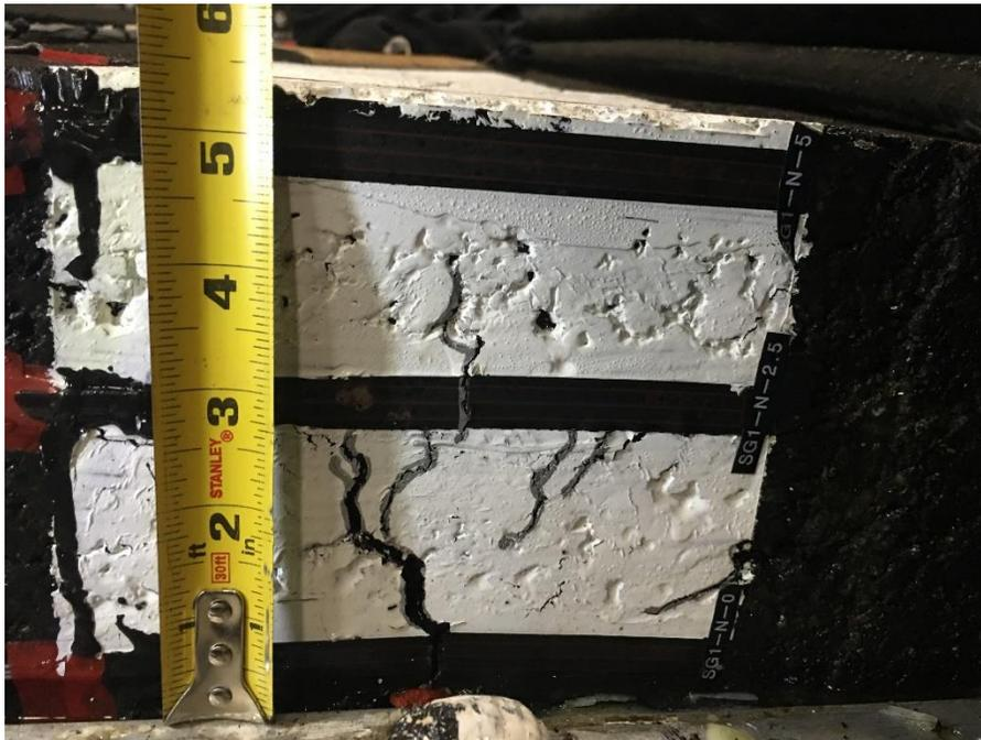
Fig 1 Bottom-up crack at SG1-N-0 and SG1-N-2.5 4.25 inch long
