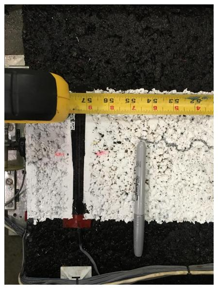
Fig 7 South section surface crack 5.5 inches from the outer vertical edge
