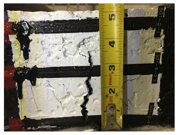
Fig 4 Bottom-up crack at SG1-S-0 3.75 inch long
