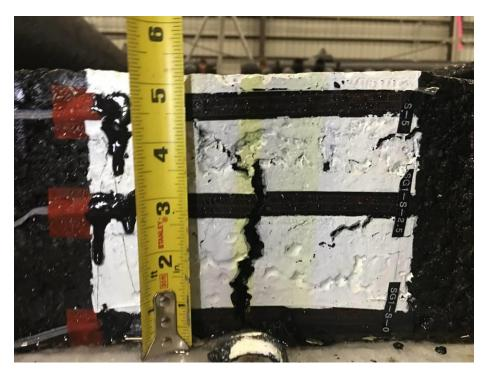
Fig 5 Bottom-up crack at SG1-S-0 4.5 inch long
