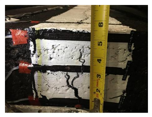
Fig 1 Bottom-up crack at SG1-N-0 and SG1-N-2.5 4.5 inch long
