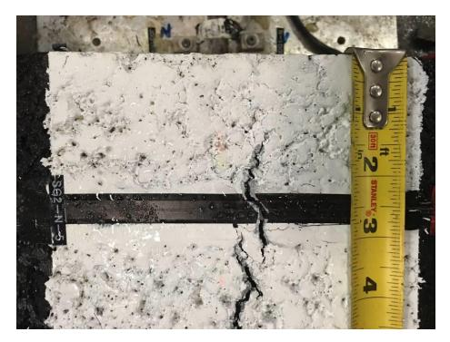
Fig 4 North section surface crack 1.5 inch from the inner vertical edge
