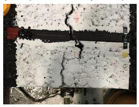
Fig 10 Surface crack on south section connected with the bottom up crack on inner edge
