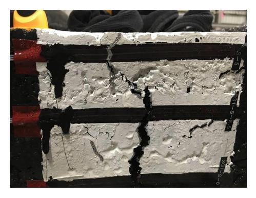
Fig 9 Bottom-up crack on south section inner edge reached the top surface
