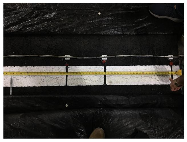
Fig 3 Surface crack on North Section approximately 7 to 56.5 inch
