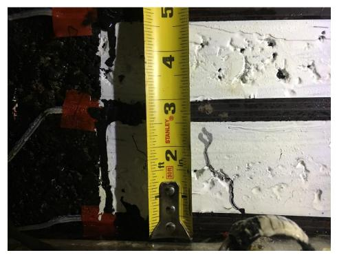
Fig 1 Bottom-up crack at SG1-N-0 2.5 inch long
