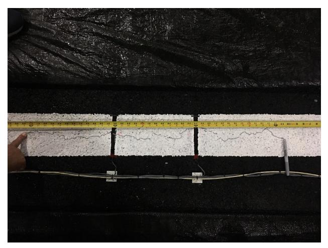
Fig 5 Surface crack on south section between 11" and 48.5"
