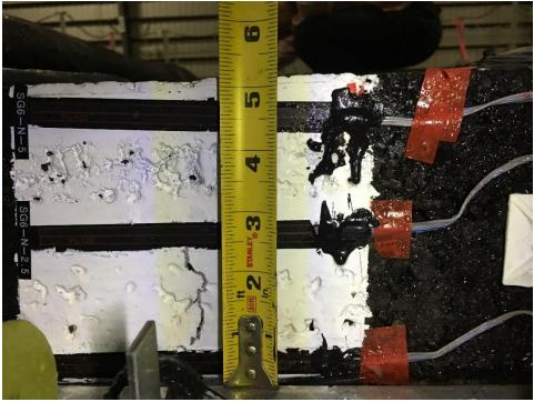
Fig 2 Bottom-up crack at SG6-N-0 2.5 inch long
