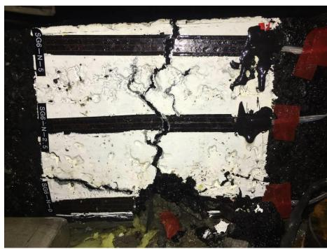
Fig 2 Bottom-up crack at north section outer edge reached top surface
