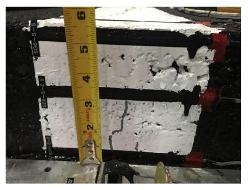
Fig 6 Bottom-up crack at SG6-S-0 3 inch long
