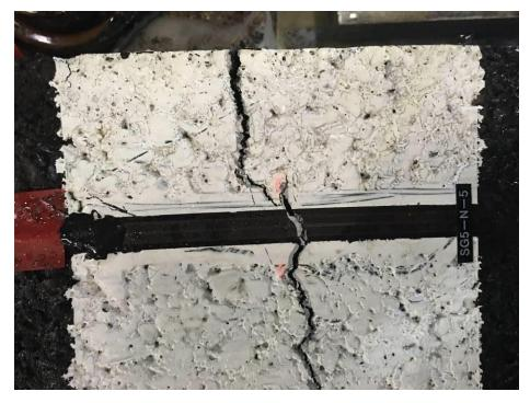
Fig 3 Surface crack on North Section reached outer edge
