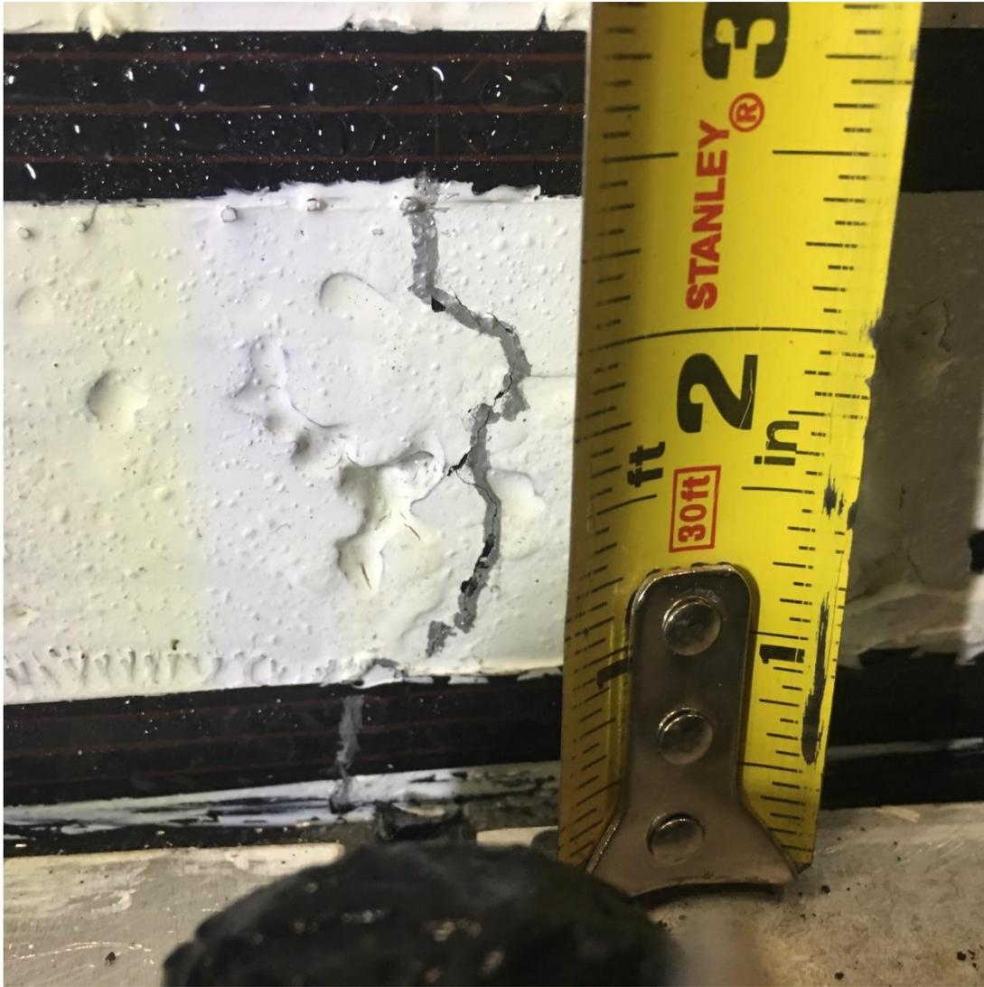
Fig 2 Bottom-up crack at SG6-N-0
