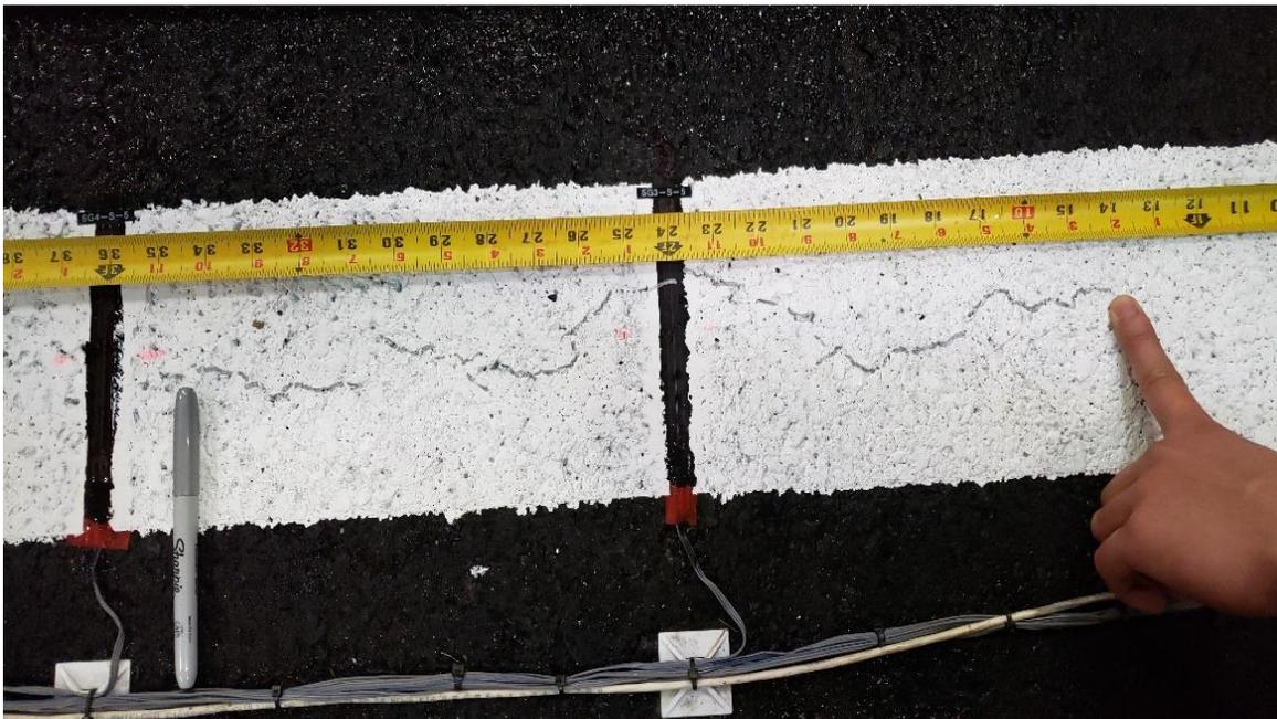
Fig 4 Surface crack on south section between 14'' and 34.5''
