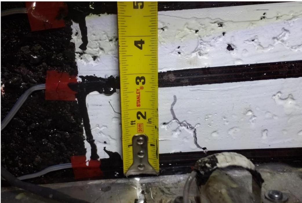
Fig 1 Bottom-up crack at SG1-N-0
