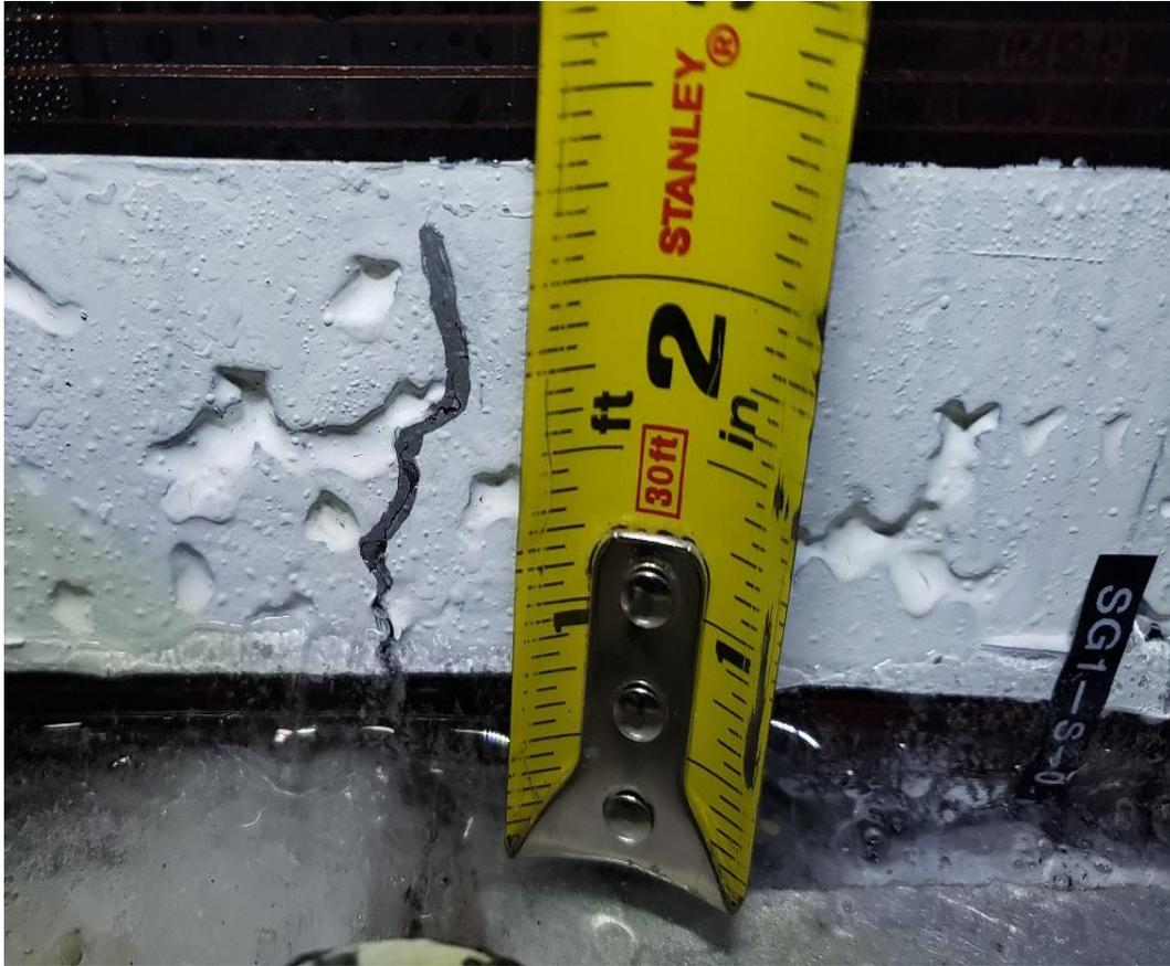
Fig 3 Bottom-up crack at SG1-S-0
