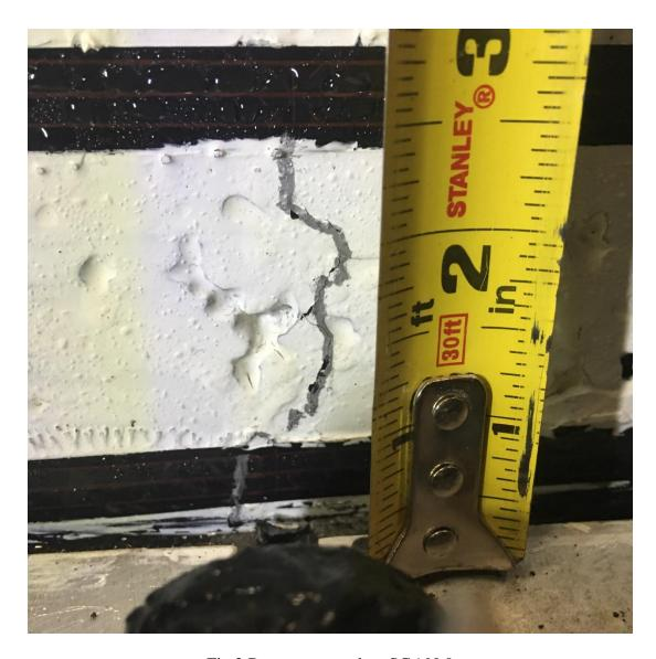
Fig 2 Bottom-up crack at SG6-N-0
