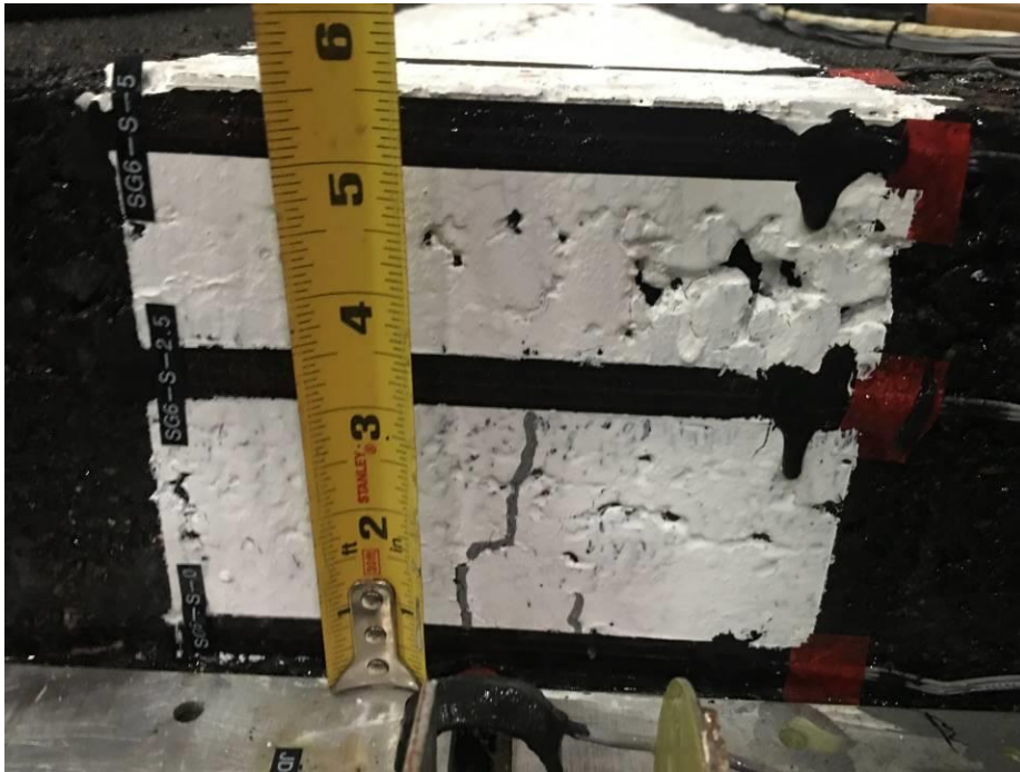
Fig 6 Bottom-up crack at SG6-S-0 3 inch long
