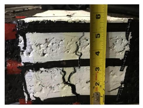
Fig 1 Bottom-up crack at SG1-N-0 and SG1-N-2.5 5 inch long
