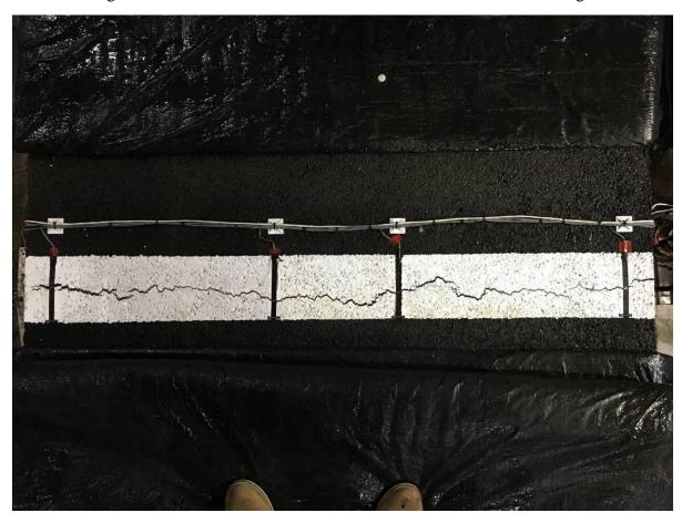
Fig 9 Surface crack on the north section
