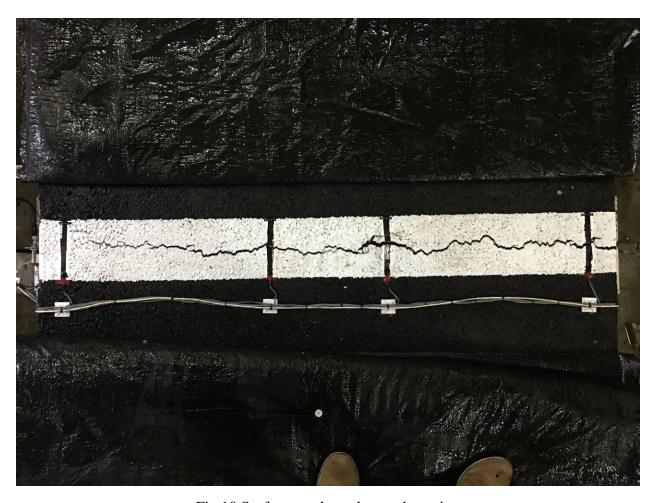
Fig 10 Surface crack on the south section
