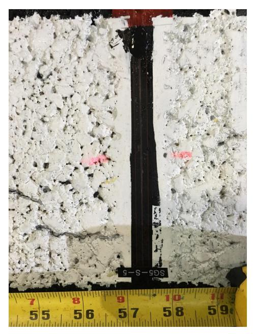
Fig 8 South section surface crack 3 inches from the outer vertical edge
