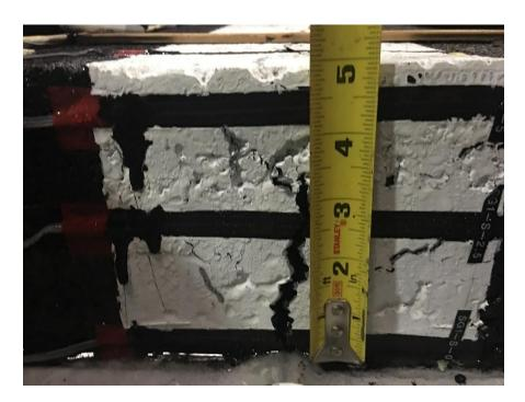
Fig 5 Bottom-up crack at SG1-S-0 4.25 inch long
