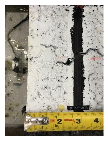
Fig 7 South section surface crack 1 inches from the inner vertical edge
