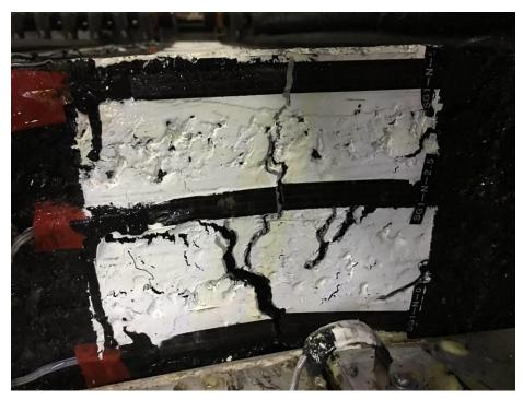
Fig 1 Bottom-up crack at north section inner vertical edge reached top surface
