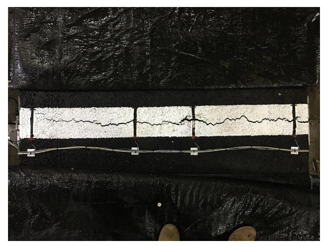
Fig 10 Surface crack on the south section
