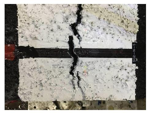
Fig 4 North section surface crack reached inner vertical edge
