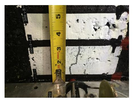
Fig 5 Bottom-up crack at SG6-S-0 3 inch long
