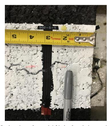
Fig 6 South section surface crack 1.5 inches from the inner vertical edge
