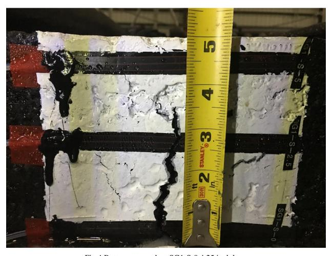
Fig 4 Bottom-up crack at SG1-S-0 4.25 inch long
