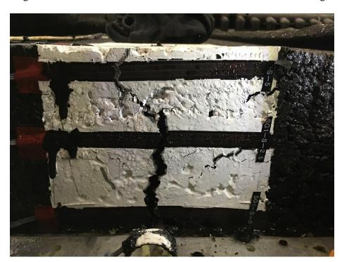
Fig 5 Bottom-up crack at SG1-S-0 reached top surface
