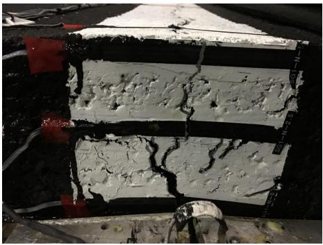
Fig 9 Bottom up crack on the inner vertical edge of North Section reached the top surface
