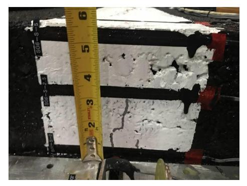
Fig 6 Bottom-up crack at SG6-S-0 3 inch long
