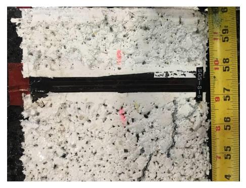
Fig 8 South section surface crack 3 inches from the outer vertical edge
