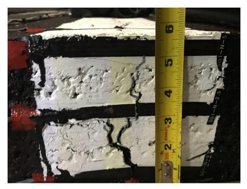
Fig 1 Bottom-up crack at north section inner vertical edge 5 inch long
