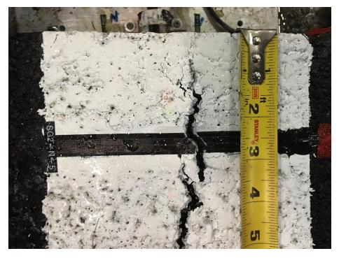
Fig 4 North section surface crack 0.5 inch from the inner vertical edge
