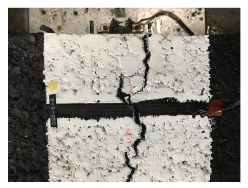
Fig 7 South section surface crack reached the inner vertical edge
