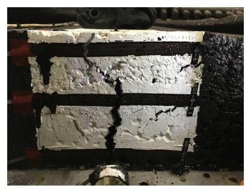
Fig 5 Bottom-up crack at inner vertical edge of south section reached top surface
