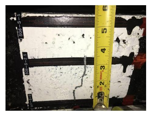
Fig 6 Bottom-up crack at SG6-S-0, SG6-S-2.5 approximately 3.5 inch long
