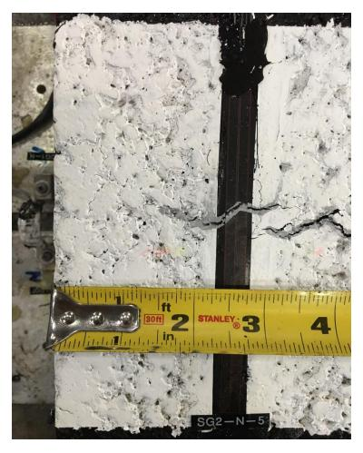
Fig 4 North section surface crack 1.5 inch from the inner vertical edge
