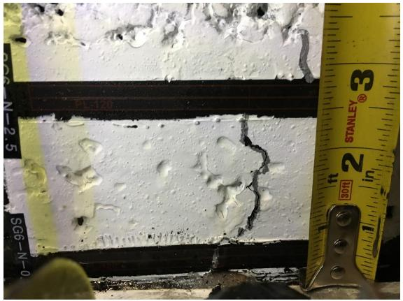
Fig 2 Bottom-up crack at SG6-N-0 3.5 inch long
