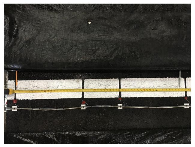
Fig 3 Surface crack on North Section approximately 4.5 to 57 inch
