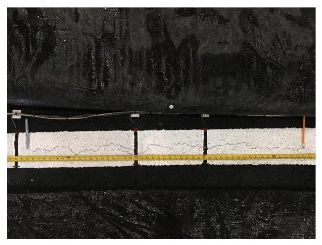
Fig 5 Surface crack on south section between 5" and 53"
