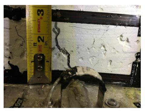
Fig 1 Bottom-up crack at SG1-N-0 2.5 inch long
