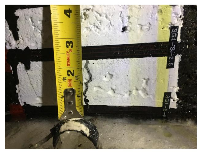
Fig 4 Bottom-up crack at SG1-S-0 2.5 inch long
